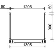
NOTE: - ALL STRUCTURE IS FULLY WELDED WITH A NOMINAL FILLET RADIUS OF 5MM.
