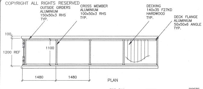
NOTE—ALL STRUCTURE IS FULLY WELDED WITH A NOMINAL FILLET RADIUS OF 5mm.
